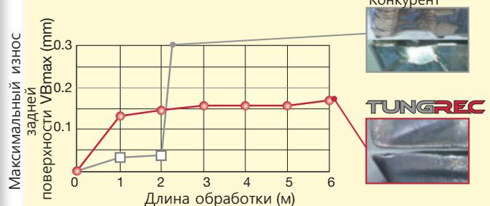
Фреза : EPO18R025M25.0-02 (ø25, z = 2, only one insert used)
